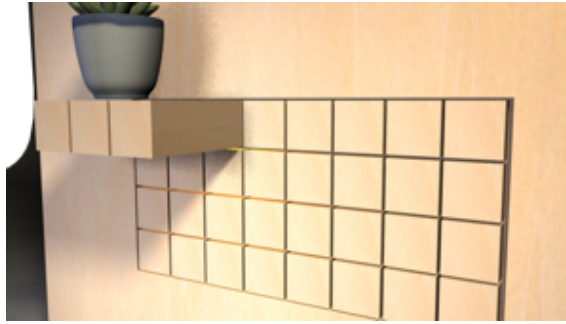
(a) The block grid inset into a wooden "wall", with three blocks extended to create a ledge and the rest at default position.
