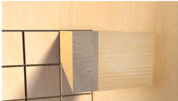
Figure 4.4: The capacitive sensor, made of a square of foil, is set under a thin wooden block face.
